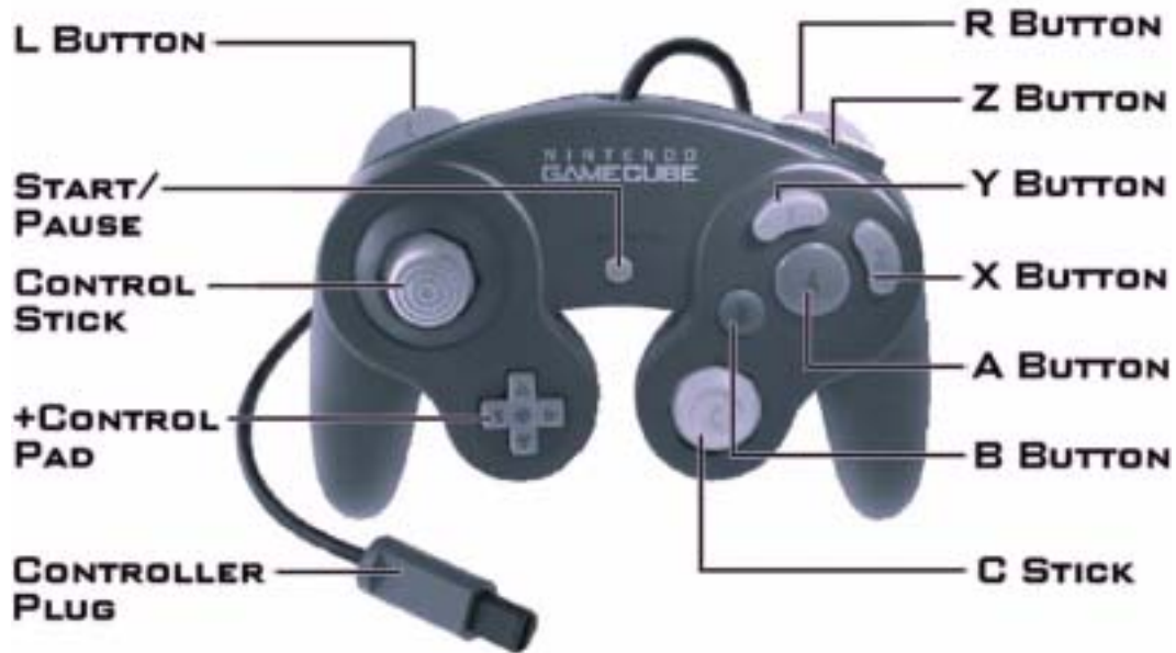
Figure 2 - Nintendo GameCube Controller Components
